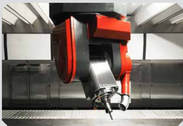
Dust Suction System on M5C milling head
