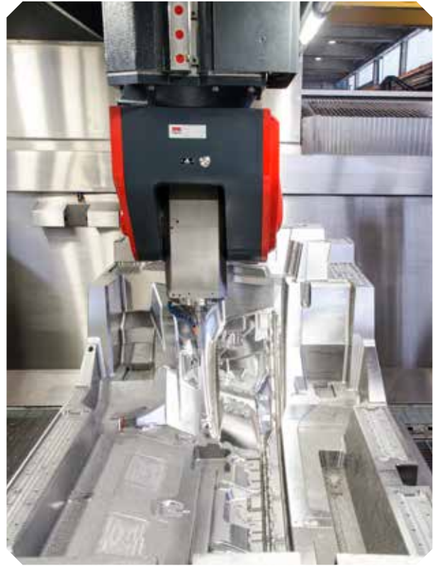
Machining of a mold for automotive industry
