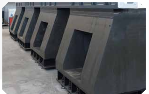
Epoxy Concrete Columns
