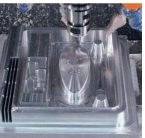
HS664 is a line of 3, 4 and 5 axis milling centres with X, Y and Z travel of 600, 560 and 400 mm, respectively.
