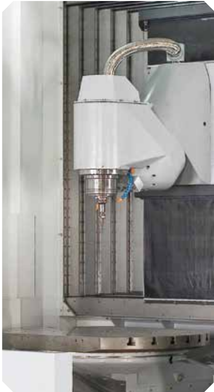
Swiveling head driven by torque motor
