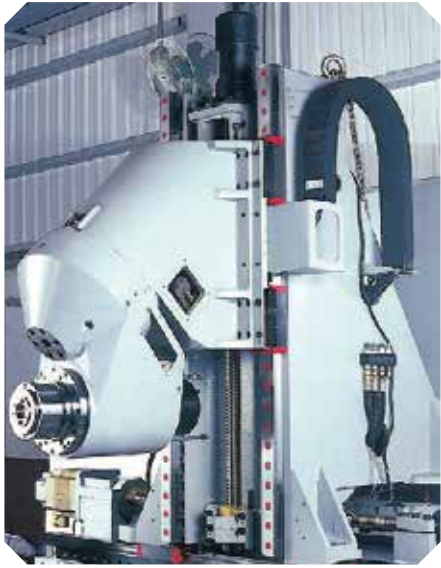
High rigid and heavy duty roller type linear guideways
