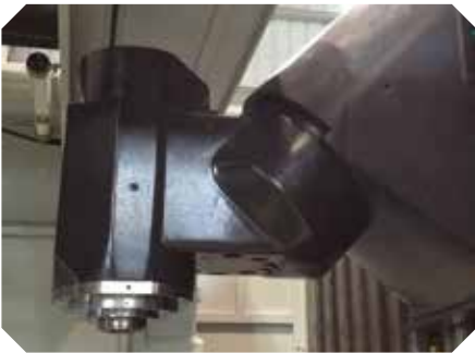
Swiveling head driven by torque motor
