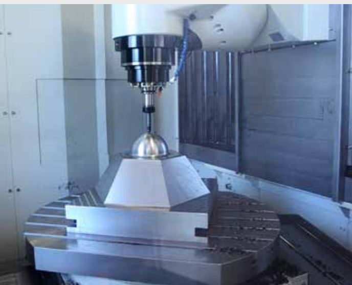
Simultaneous 5-axis high accuracy machining
